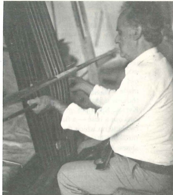
A shepherd's bag being woven on the vertical loom which can also be used for making rugs.
